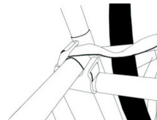
4. USE STRAP (NOT INCLUDED) TO PULL ALL BICYCLES TOGETHER AROUND BOTTOM BRACKETS. STRAP SHOULD ALSO SECURE WHEELS.
